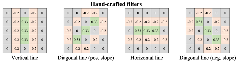
Figure 6.3: The hand-crafted filters of the sensory system are used to extract features from the images. The filters are optimised for horizontal, vertical, and diagonal lines.
